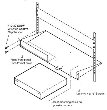
Figure 2 — Rack mounting the CVC 200
